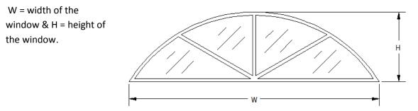
Find the radius of an arch window accurate to the 16<sup>th</sup> of an inch, which has a width of 42 inches and a height of 12 inches.
