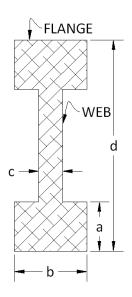
Note: Moment of inertia is a measure of a beam's effectiveness at resisting bending based on its cross-sectional shape.
